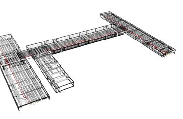
Full structural loading and lifting calculations are used to determine lifting and fixing points for each module, while detailed BIM coordination enables seamless onsite positioning and installation. Once installed, we fabricate spool pieces for connection between each module, prior to final testing on site.
